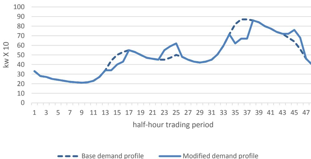
Figure 1. A Domestic Customer's Demand Profile Modified in Order to Provide a Balancing Service<sup>3</sup>
