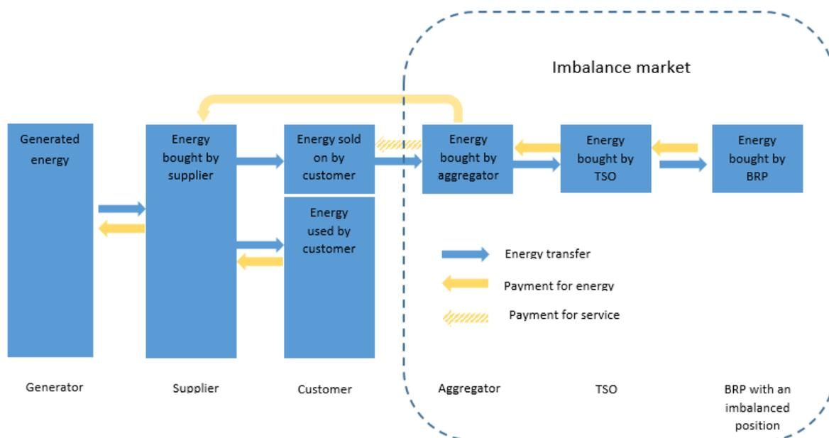
**Figure 2. Energy Flows and Payments When an Aggregator Decreases a Customer's Demand as Part of a Flexibility Service**
