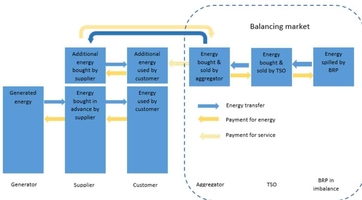
Figure 3. Energy Flows and Payments When an Aggregator Increases a Customer's Demand as Part of a Flexibility Service
