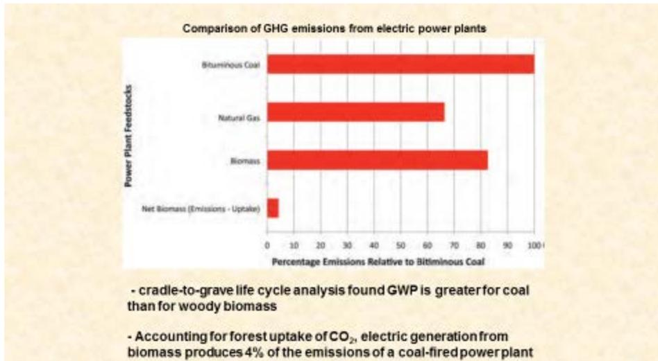
**Figure 8. Biomass GHG Emissions vs. Fossil Fuel Sources**
