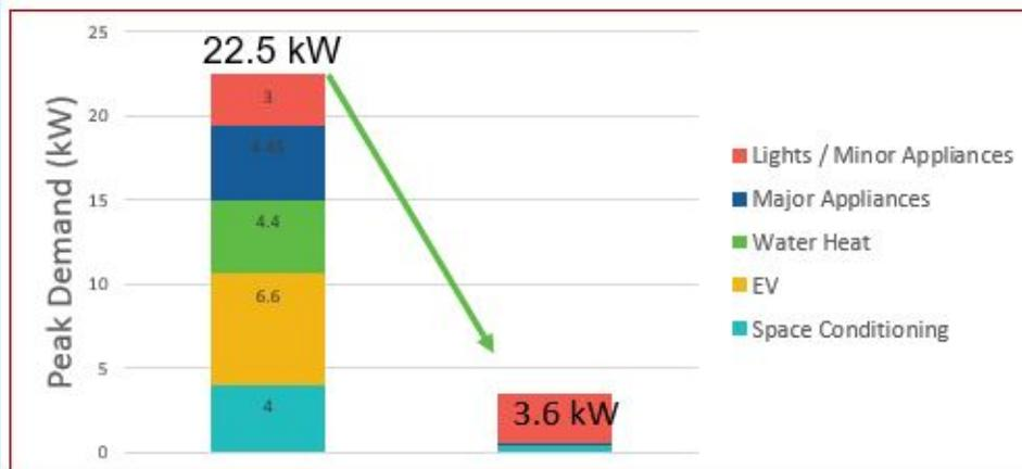
Electric vehicles are another form of controllable load. A level 2 charger would contribute about 6.6 kW to peak demand if not controlled.
