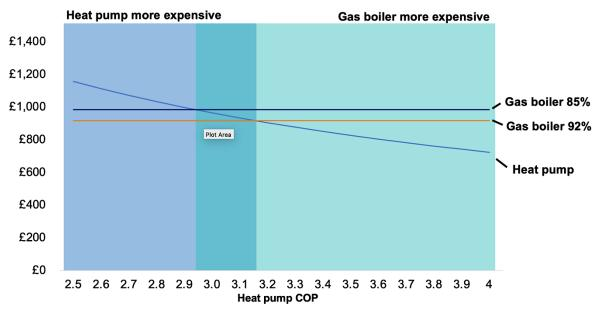
Assumptions: Heat demand: 10,204 kWh; Cost gas: 7.37p/kWh; Cost electricity: 28.34p/kWh; Gas standing charge: £0.27/day
