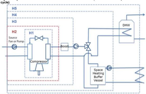
Figure 4. System boundaries used for COP/SCOP calculations (NB: 'Boost' is for pasteurization
