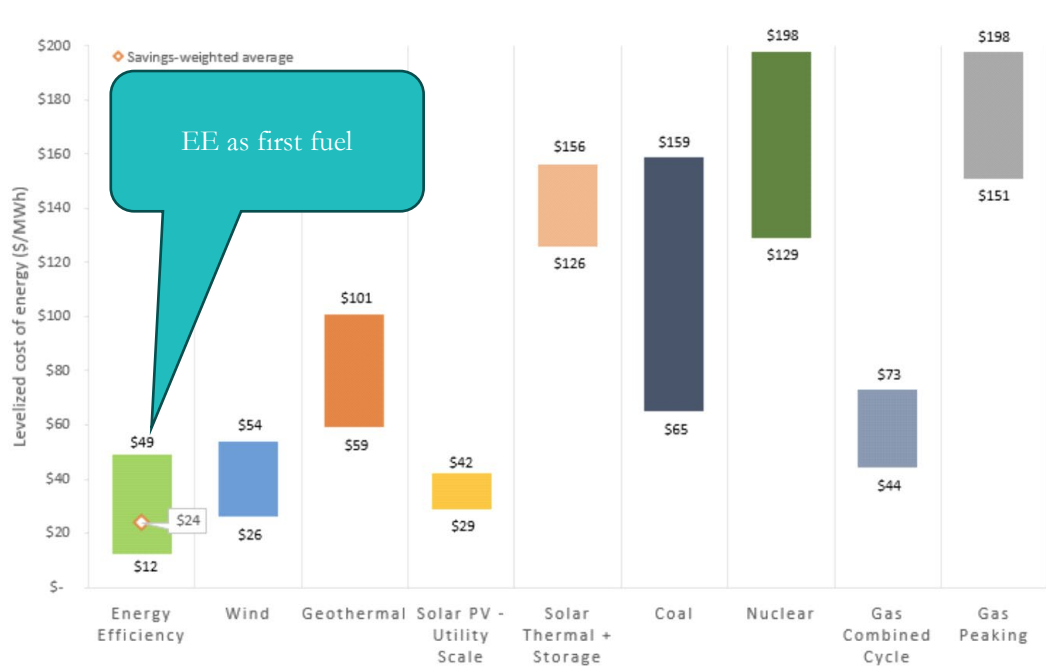
Figure 2. Energy efficiency interventions are lowest-cost resource
