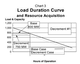
Now the peak load requirement for the utility is 950 MW, and the minimum load requirement is 250 MW. Again, by drawing a line from 2500 hours to intercept the new load curve, it can be seen that, despite the free MW, 200 MW must still be acquired to meet the load requirements for 2500 hours of the year. On the other hand, now only 750, not 800 MW are needed to meet the base-load requirements.
