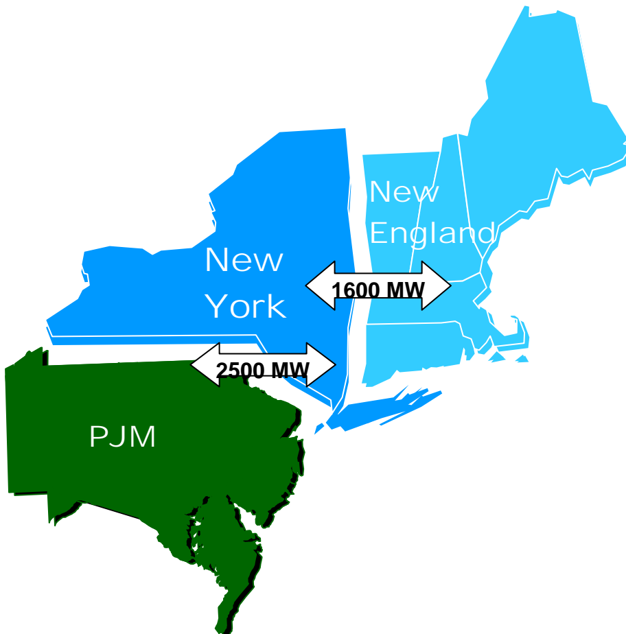
Figure 1: Three regional systems in the Northeast U.S. with transfer capacities noted. Source Remarks of Gordon van Welie to FERC, March 13, 2002.
