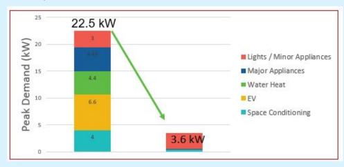
Electric vehicles are another form of controllable load. A level 2 charger would contribute about 6.6 kW to peak demand if not controlled.
